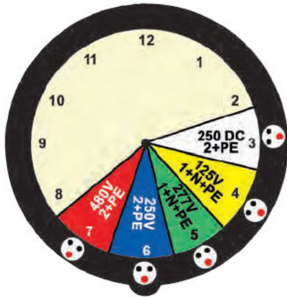
3 wires: 2+PE & 1+N+PE
