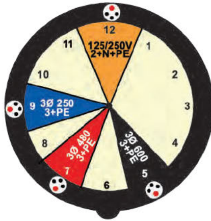
4 wires: 2+N+PE & 3+PE
