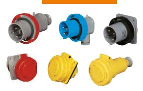
EPIC® CEE and MULTIMAX series pin & sleeve connectors handle single phase and three phase power requirements up to 600 volts and 125 amps. MULTIMAX connectors can be assembled in under 20 seconds, and an innovative retaining tab prevents unintentional withdrawal by engaging with the mating connector's cover.
