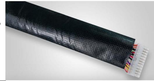
**Material Type PVC-coated polyester Operational Temp** -40° to 179.62°F | -40° to 82°C 120 lbs/min (warp) | 100 lbs/min (fill) **Tensile Strength** Fluid Resistance Hydro resist - 150 psi **Material Thickness** 0.010" Flame Retardant FED-STD-191 method 5903 Mil-Spec MIL-C-43006G, type II, class 1 **Flexibility** ★ ☆ Better **Color Options RoHS Compliant** Yes Specifications are based on finished product attributes
